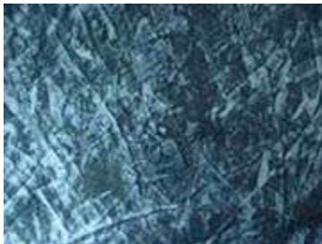
Photo 10: A busy finish attained by using the sharp edges of the blades.
